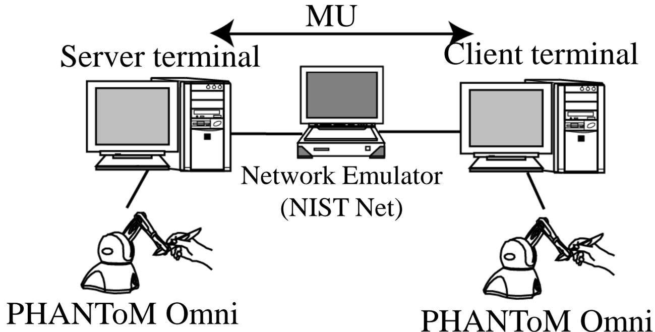
**NIST Net generates an additional delay for each MU transmitted between the client and server terminals.**
