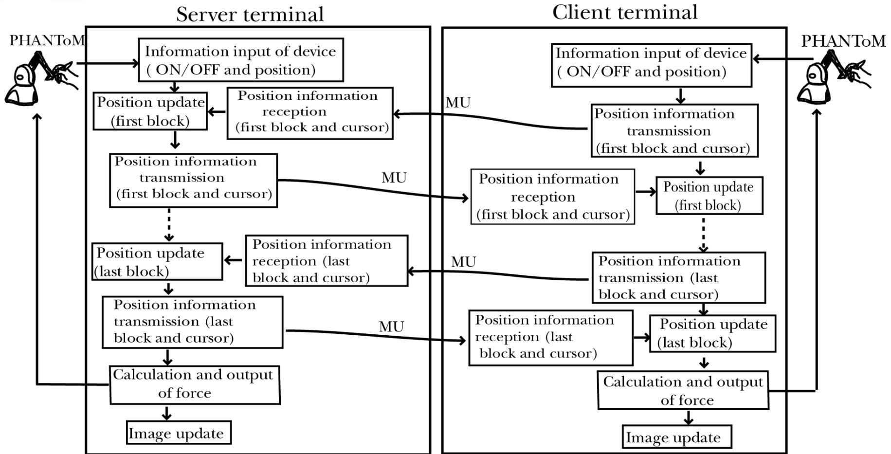
The client and server terminals transmit a stream of MUs, each of which includes the sequence number, the information about the stylus button (ON/OFF), and the position information of the  $i$ -th block.
