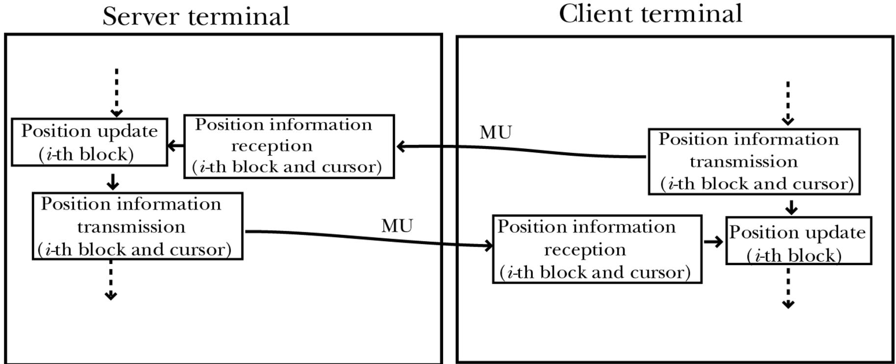
When the server terminal updates the position of the  $i$ -th block, the position of the block is set to the middle between the position of the server terminal's  $i$ -th block and that of the client terminal's  $i$ -th block. The client terminal updates the position of the  $i$ -th block by using the position information which is transmitted from the server terminal.
